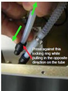
Press against this locking ring while pulling in the opposite direction on the tube
