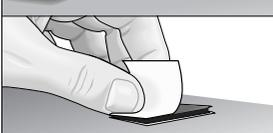
4. Attach the detector to the hook-and-loop fastener. You can remove and reattach the unit as often as you like.
