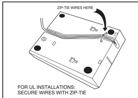
Figure 3. Securing Wires
