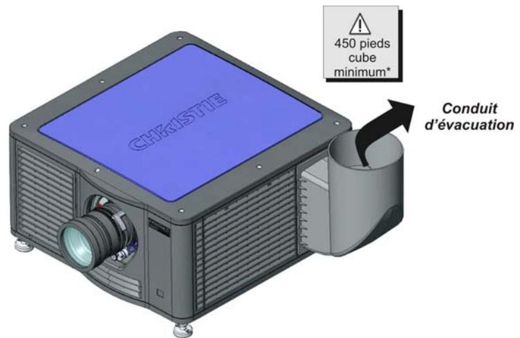
SCHÉMA 3.3 CONNEXION DU CONDUIT
