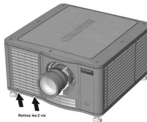
SCHÉMA 4.2 REMPLACEMENT DU FILTRE
