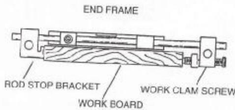
6. Loosen the wing nuts on the rod stop brackets and slide both brackets up against the rear of the work board. (Retighten wing nuts).
