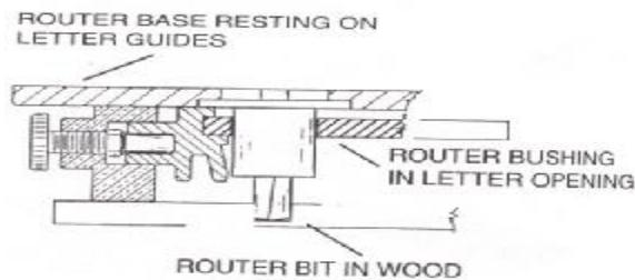
8. Review the safety rules in router owners' manual. With router electrical cord unplugged, install router bushing and router bit. Set router bit 11/16" below router base for your first sign. This will give 3/32" deep engraving.
