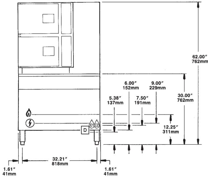
**NOTE:** When ordering optional reverse door openings: Control Panel, door openings, and cooking compartments are located opposite that shown above and positioned on right hand side of base.
