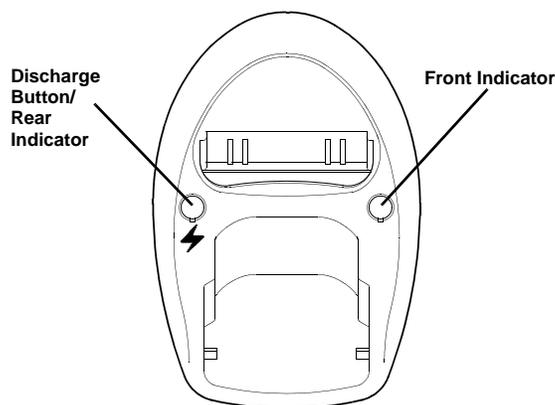
2. To charge a battery that is installed in a Nokia 5100 or 6100 cellular phone, insert the phone into the charger's front chamber. The red indicator lights. The indicator does not change, since charge status is indicated by the phone.
