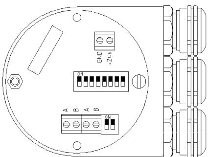
Connect the Power supply (switched OFF!) on the GND and +24V
