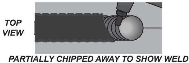
Slag is a necessary part of a flux-core wire weld. It shields the weld from impurities. Clean off the slag with the Chipping Hammer and Wire Brush after welding.
