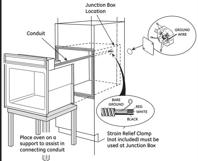
**B3** This oven is supplied with a 123 cm (48") long flexible conduit consisting of:
