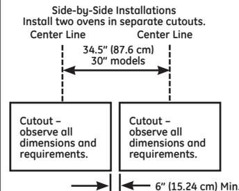
If the cabinet does not have a solid bottom, two braces or runners must be installed level with the bottom of the cutout to support the weight of the oven. For single ovens, the runners and braces must support 68 kg (150 lbs.).
