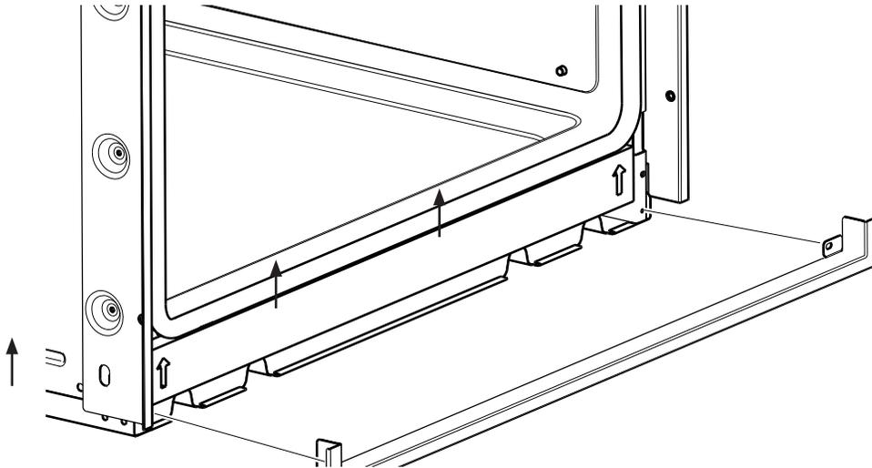
**IMPORTANT:** If this unit is ever removed from the cabinet or the oven is ever pulled out for service, the bottom trim must be removed first or damage to the trim will occur.
