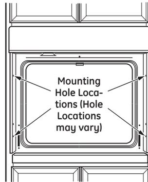
The screws must be a minimum of 6 mm (1/4") from the front of the cutout.
