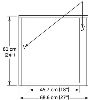
**NOTE:** If marks, blemishes or the cutout opening are visible above the installed oven, it may be necessary to add wood shims under the runners and front trim until the marks or opening are covered.
