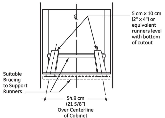
**NOTE:** If marks, blemishes or the cutout opening are visible above the installed oven, it may be necessary to add wood shims under the runners and front trim until the marks or opening are covered.
