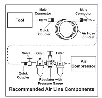
Incorporate an in-line oiler, shut-off valve, regulator with pressure gauge, and filter for best service, as shown in the diagram above. An in-line shutoff valve is an important safety device because it controls the air supply even if the air hose is ruptured.
