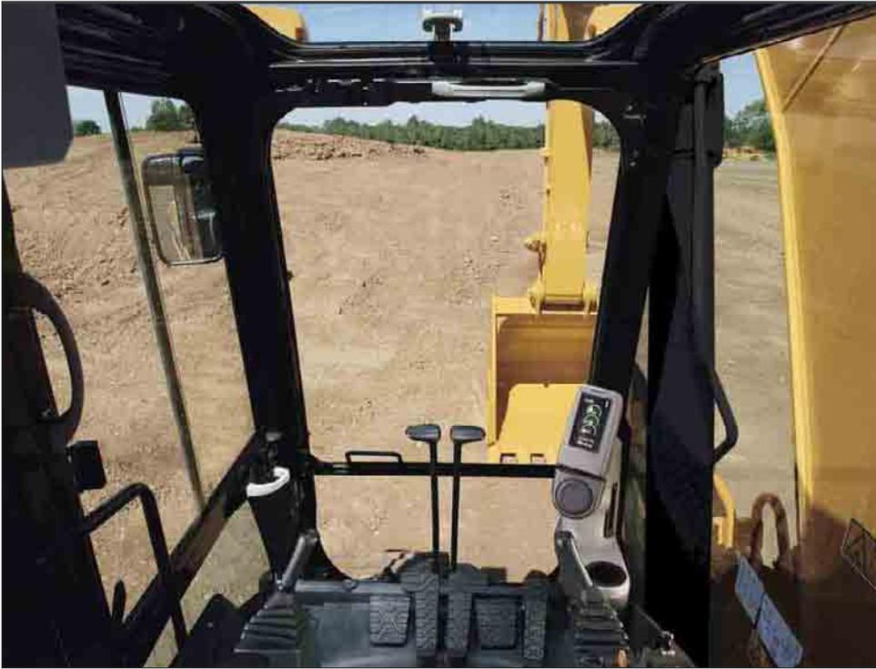
**Operator Station.** The workstation is spacious, quiet and comfortable, assuring high productivity during a long workday. The air conditioner and attachment switches are conveniently located on the right-hand wall, and the key switch and throttle dial are on the right-hand console. The monitor is easy to see and maximizes visibility.
