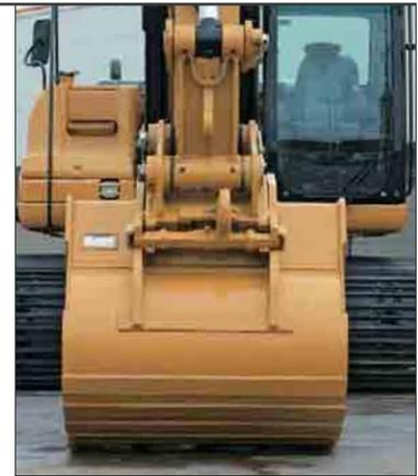
**Bucket Linkage.** Two bucket linkages (CB2 and DB) are available, with lifting eye on the power link.
