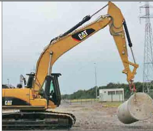
**Heavy Lift Mode.** Maximizing lifting performance and boosting the lifting capability. Heavy loads can be easily moved in the full working range of the machine maintaining excellent stability.
