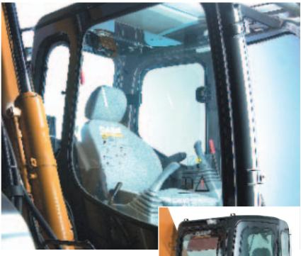
the attachment is fully retracted. For operator comfort, the cab is insulated from vibration and noise by four elastofluid mountings.
