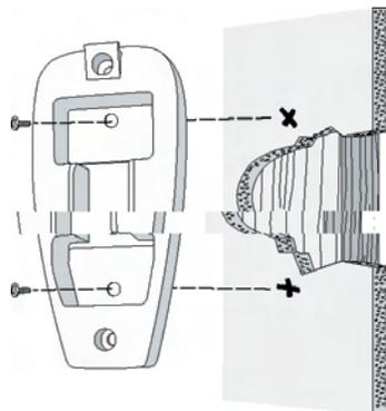
**NOTE:** The wall anchors and 6-32 x 1" screws may be used in situations where mounting to a stud is not possible. Use the inner mounting holes. After securing the anchor, discard the anchor's pointed screws and use the 6-32 decor ovalhead screws supplied.
