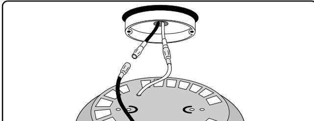
*NOTE: International fans and light fixtures are supplied with plug and socket connectors. Substitute these connectors for the wire nuts shown throughout this manual.*
