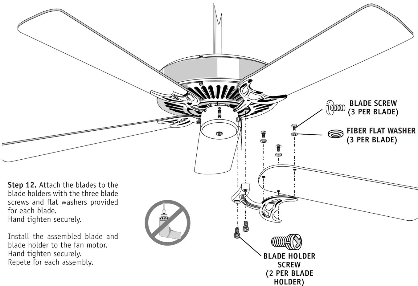
**Step 12.** Attach the blades to the blade holders with the three blade screws and flat washers provided for each blade.
