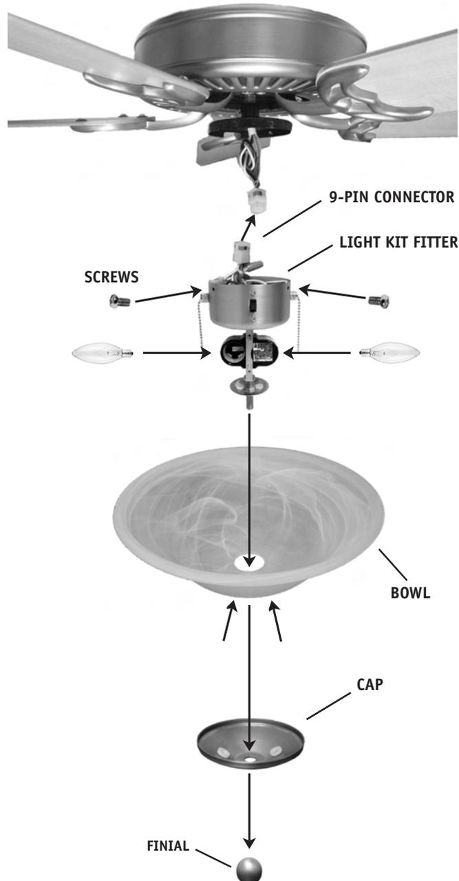
**Note:** In compliance with US Federal Energy Regulations, this ceiling fan contains a device that restricts the light kit to a maximum of 190 watts. Exceeding that limit or the marked limit on this product may result in fire hazard or improper operation.
