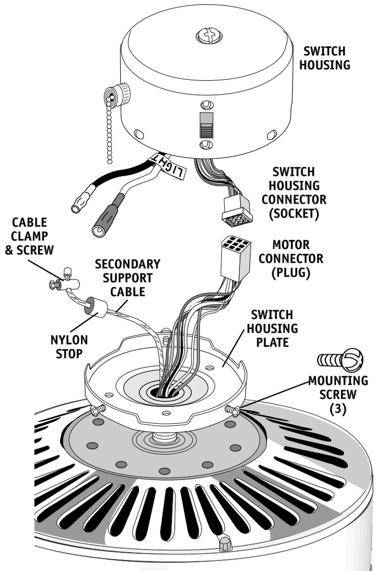
**OUTSIDE USA - SECONDARY SUPPORT ♦ SWITCH HOUSING INSTALLATION**
