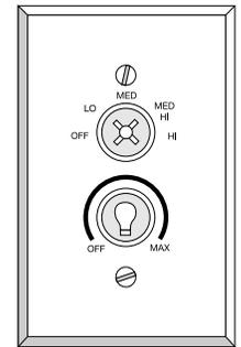
**CAUTION! Failure to set the pull-chain speed to HIGH can result in faulty operation of the fan and damage to the W-8 wall control. To confirm fan is set to HIGH: Turn W-8 fan speed switch to 'HI' - set fastest fan speed with pull chain.**
