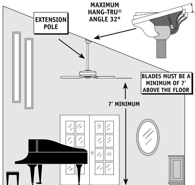
*Note: Fan may wobble or vibrate if pole length is not long enough and inside blade is too close to downslope or side wall. Extending pole length will usually solve problem.*
