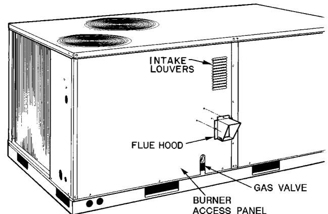
Fig. 1B — Gas Valve Location (Sizes 008-014)
