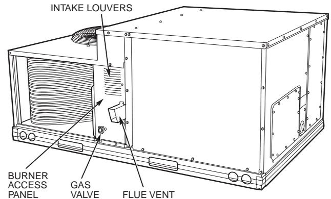
Fig. 1A — Gas Valve Location (Sizes 004-007)
