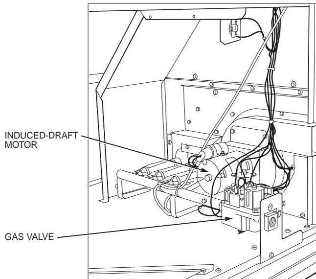
**Fig. 5 — Typical Heat Section Detail (Size 004-007 Shown)**
