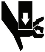
Pinch point hazard. Crimp ram operates at high speed and force and can cause severe personal injury. Keep all body parts away from moving parts of the tool, especially the T-track area of the head and die holder during operation.
