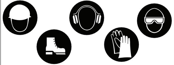
Use all appropriate personal safety equipment when handling, operating, and servicing this tool such as: safety shoes, hard hat, eye and ear protection, work gloves, and sleeves.
