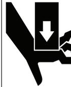
Pinch point hazard. Crimp ram operates at high speed and force and can cause severe personal injury. Keep all body parts away from moving parts of the tool, especially the T-track area of the head and die holder during operation.
