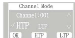
**ATTENTION:** HTP: higher value output first. LTP: the signal of the controller output first. If you want to set most channels to HTP, you can first choose "ALL CH HTP" then enter article 3 to retrigger separately, and vice versa.
