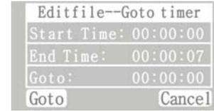
3. Turn the jog wheel to adjust the start time, then press "Goto" button to store, or press "Cancel" button to exit without any change.
