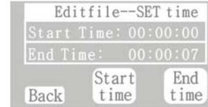
4. In edit mode, press "Timeset" button to set start/end position. Press "Start Time" button and use the jog wheel to adjust the start time ( default start time is 00:00:00), after setting, press "Save" button to store, or press "Cancel" button to exit without any change.
