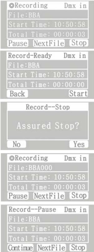
Press the “Start” button to start real time DMX records, “Recording” will be blinking. In order to save memory space, the total time will not change if there is not any DMX input. DMX signal clue will show in the upper right.
