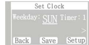
3. You can set timer week, timer number, startup hour, startup minute, startup second, shutdown week, shutdown hour, shutdown minute, shutdown second, run time, timer on or not. Press "Setup" button to setup. You can set a maximum of 21 timers a week, 3 timers per day.
