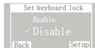
3. Press "Setup" button to setup, turn jog wheel to change play mode (1.Enable 2.Disable), press "OK" button to confirm.
