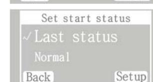
3. Press "Setup" button and turn jog wheel to change the start status (1.Master 2.Slave), press "OK" button to confirm, or press "Back" button to exit without any change.
