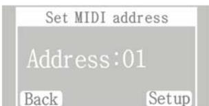
3. Press “Setup” button, and turn jog wheel to adjust the MIDI address.
