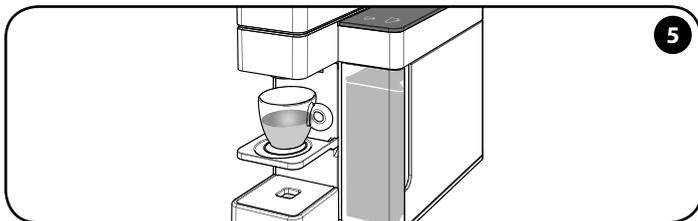
The new setting is saved. The machine is now programmed; the next time the ☕ button is pressed, the programmed quantity of coffee will be brewed.
