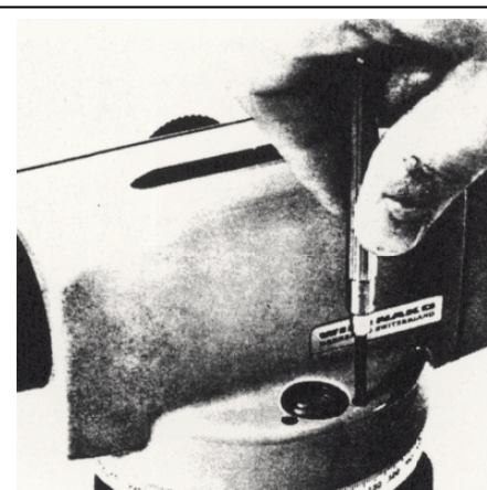
Figure 19: Wild N2 (direct image) – circular bubble adjustment
