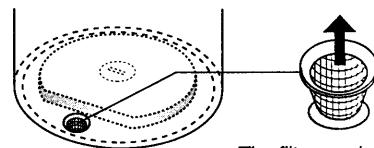
The filter can be removed by pulling firmly on it.
