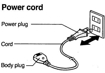
15. Do not allow small metal parts near the body plug.
