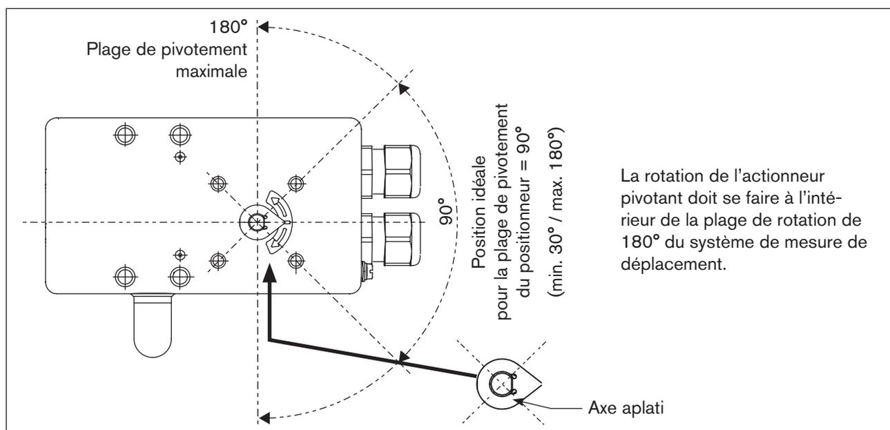
Figure 27 : Plage de rotation / Protection anti-torsion
