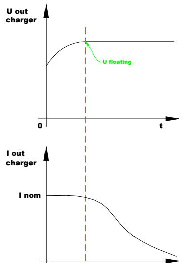
With this setting, the CPS3 charger produces a single-stage UI type load curve. It generates a constant voltage, supplying the current required by the battery(ies). Recharging time depends on the state of the battery, being longer than when the boost is in the ON position.
