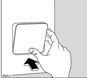
Open the filter door and place a container underneath to catch any spillage. If the filter is blocked and the machine is unable to drain you will need to drain the water manually from the machine at this stage. To do this, unhook the drain hose from the
