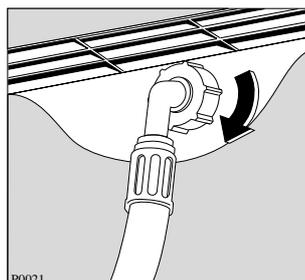
Set the hoses correctly by loosening the ring nuts. After positioning the inlet hoses, be sure to tighten the ring nuts again to prevent leaks.
