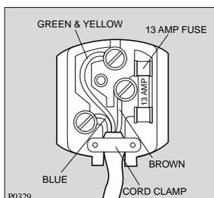
Connect the green and yellow (earth) wire to the terminal in the plug which is marked with the letter «E» or the earth symbol  $\perp$  or coloured green and yellow.
