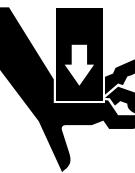
Pinch point hazard. Crimp ram operates at high speed and force and can cause severe personal injury. Keep all body parts away from moving parts of the tool, especially the T-track area of the head and die holder during operation.
