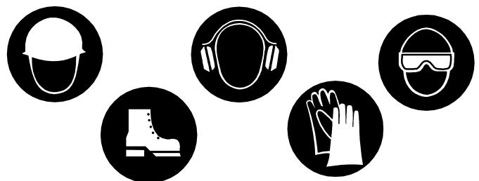
Use all appropriate personal safety equipment when handling, operating, and servicing this tool such as: safety shoes, hard hat, eye and ear protection, work gloves, and sleeves.
