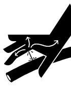
Hydraulic fluid under pressure. Do NOT use any part of your body to locate a hydraulic leak. Escaping fluid under pressure can cause severe injury or death. If injury results from escaping hydraulic fluid, seek immediate medical attention to avoid serious bodily injury.
