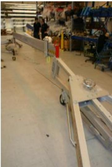
Figure 1: Beam and A-Frames positioned for assembly
