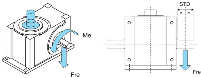
Fre = Forza radiale entrata (N)/ Input radial force (N)/Radialkraft Antrieb (N)/ Force radiale en entrée (N)/ Fuerza radial de entrada (N)
