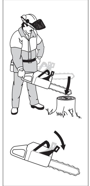
When the bar hits the stump the brake should be applied.
