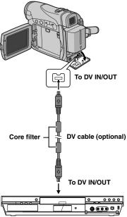
Video unit equipped with DV connector
