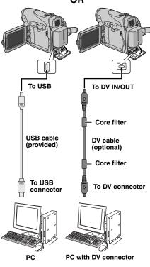
When connecting the camcorder to a PC using a DV cable, make sure to follow the procedure below. Connecting the cable incorrectly may cause malfunctions to the camcorder and/or the PC.
