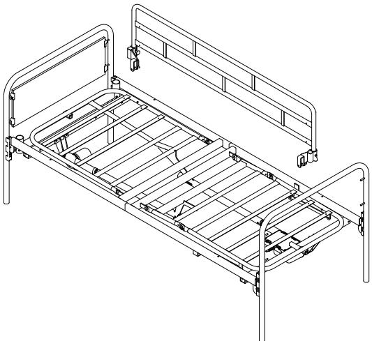
Place the side rail on the frame close to the front bed end.
