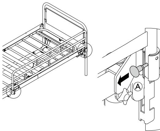
Pull out the locking pins on both sides and push the side rail down, slowly.
