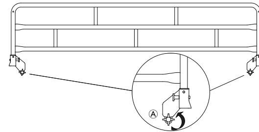
Loosen the knobs A on both attachments on the side rail.
