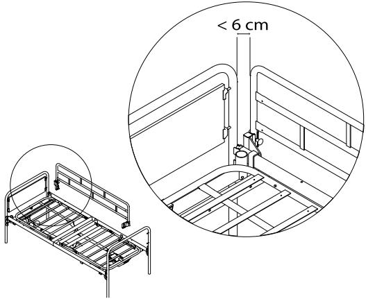
Lower the side rail onto the front leg attachment and tighten with the knob.
