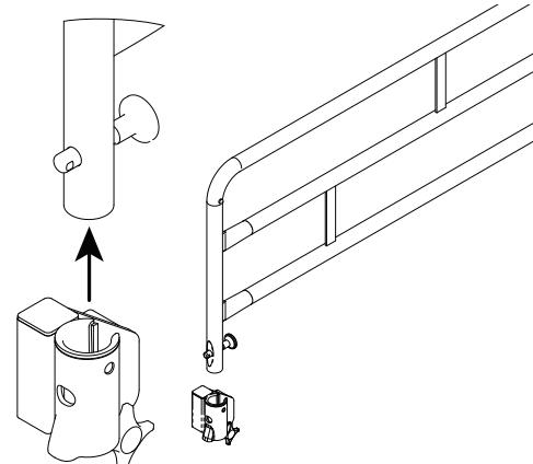
Pull out the pin and mount the bracket on the side rail. Make sure that the pin locks the bracket and that the hand wheel is on the outside of the side rail.
