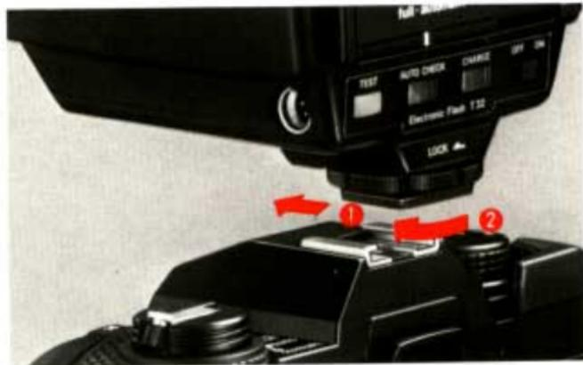
Slide the flash into the camera's accessory shoe and lock it by turning knob until the flash is tight. Make sure the flash is pushed fully forward, to insure proper electrical contact.
