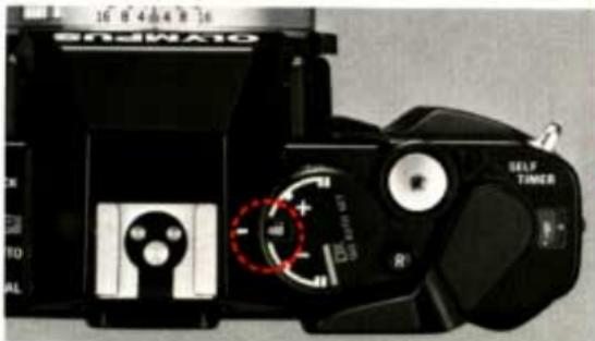
**E** If the film speed dial (exposure compensation dial) cannot be turned to the ISO number of the film used, set it once at an intermediate value then repeat steps 2 to 3 until the desired ISO number is set.
