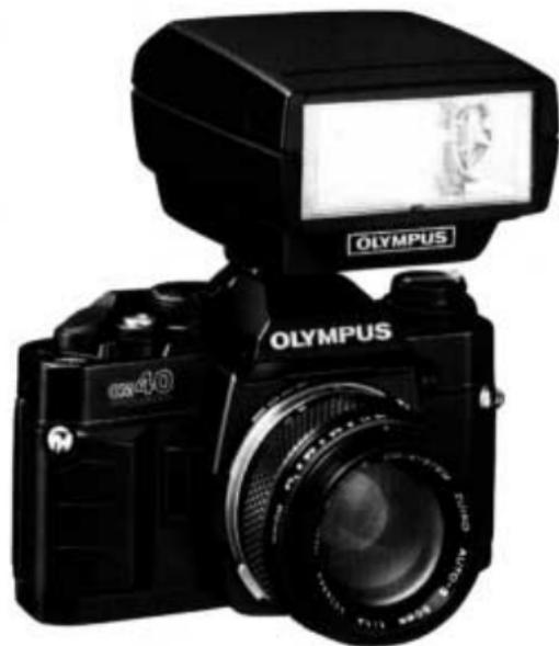
The OM-40 PROGRAM is designed to provide "OTF" Automatic Exposure with Olympus T-Series electronic flashes. There is nothing to set since exposure is determined by the sensors in the camera body itself. You can even adjust exposures using the compensation dial on the camera. Because it directly measures the light at the film plane, it does not allow for flash exposure error utilizing the sensor built into the flash.
