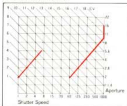
The OM-40 PROGRAM assures you "OTF" Program Auto flash performance when you use an OM System T Series flash unit. The flash will fire automatically at program shutter speeds of 1/60 sec. or slower, whenever the flash unit is switched ON. In this situation the camera program automatically shifts three settings to the special Flash Program. The final exposure is made precisely accurate by the camera computer; which shuts off the flash the instant the right amount of light has reached the film.
