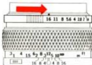
**E** If the shutter speed is too slow, set the aperture to smaller number to prevent camera shake.
