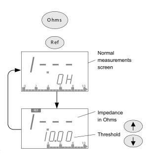
and the bottom line shows the reference level. Adjust the reference level by using the Up and down arrow buttons. Now when the impedance is below the reference value, you should hear a beep. The reference value is set for a particular range – you may need to readjust it for a different range. The reference value will be saved in the internal memory.
