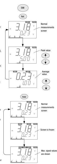
is active. Please note that if you power down the  $3M^{\infty}$  Ground Pro Ground Integrity Meter while in any of these modes, it will remain in the same mode when the unit is powered up again.
