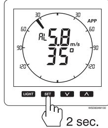
When the alarm is switched on **AL** will be displayed when in normal display.
