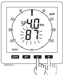
The original value can always be reset by pressing the **LIGHT (RESET)** button.
