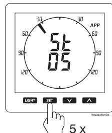
The wind direction is shown by the number of segments from '0' (scale is 2x 70°, 'Close Hauled') and in degrees from '0'.
