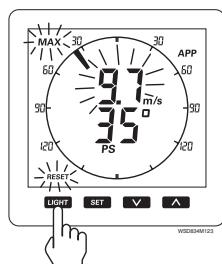
After pressing the **LIGHT (RESET)** button the maximum wind speed since the reset will be displayed.
