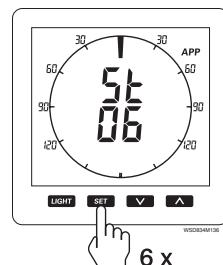
The ship's speed will be displayed, always in knots, together with the calibration figure as a %.
