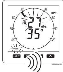
The alarm can be suppressed by pressing the **LIGHT** (**RESET**) button.
