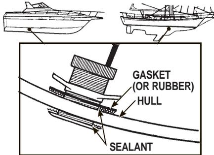
7. Put the nut on the transducer from the inside of the hull. If nylon, hand tighten only.
