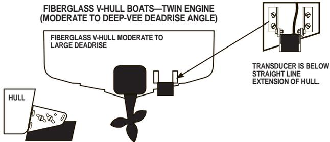
**DO NOT** INSTALL YOUR TRANSDUCER UNDERNEATH A GASOLINE OVERFLOW. THIS WILL DESTROY THE PLASTIC MATERIAL OF THE TRANSDUCER AND THE BRACKET. THIS DAMAGE IS NOT COVERED UNDER WARRANTY. Also, **do not** use LOCKTITE® or any other solvents on the mounting hardware or transducer. These materials may destroy the transducer.
