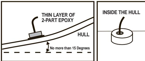
When the epoxy has cured, it should be permanently bonded to the hull and hard to the touch. Test the epoxy which extends out of the underside of the transducer with a screwdriver to ensure that it can't be dented, and that it is completely hard. *Epoxy which is not hardened will eventually cause improper readings.*
