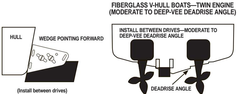
3. Mark the outline of each slot on the hull. Mark the screw locations 1/8" from the *bottom* of each slot, and drill four holes 3/4" deep with a 9/64" drill. The slots in the bracket allow 5/8" of vertical adjustment which can be utilized to lower the transducer further into the water to achieve optimal performance.
