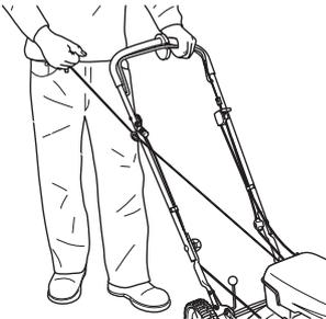
**CAUTION!** Do not pull the starter cord all the way out and do not let go of the starter handle when the cord is fully extended. This can damage the machine.
