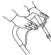
The brake handle must never be permanently anchored in handle when the machine is running.
