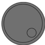
The **knob** (double function rotation and key press) allows to choose the parameter to be modified (by rotation), if it is a numerical value or a name to select or unselect (by key press) and to modify it (by rotation). It can be associated the soft keys <- and -> to select the figure or the letter to be modified.
