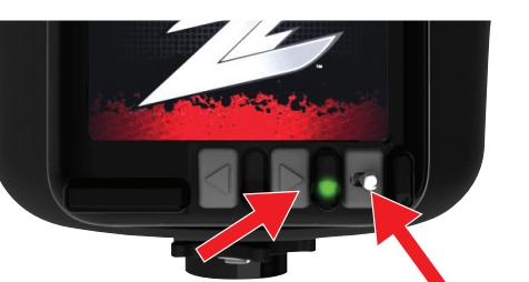
**Loader Operation -** The Empire Prophecy Z2 loader is activated by sound and sensors. Simply turn the Z2 on and you're ready to go. The Z2 will pickup the sound of each shot fired and use its sensors to feed paintballs to your marker. No adjustments are needed.
