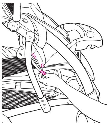
Undo snap and unfasten hook and loop strap on each side of the stroller.
