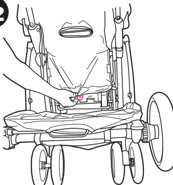
Unhook plastic tab on underside of the back of seat base.
