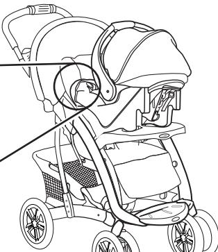
• **To unlock restraint latches:** Push release button beneath the restraint latch and rotate away from infant car seat.
