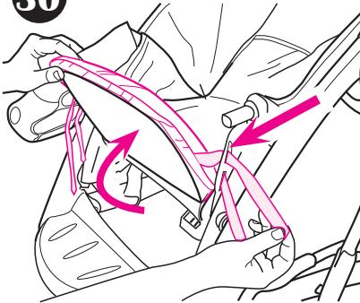
Open child's tray, lift enclosure, and thread straps through button holes on each side of seat cover.
