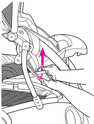
Unhook plastic tabs on each side of seat bottom, and pull straps out of slots.
