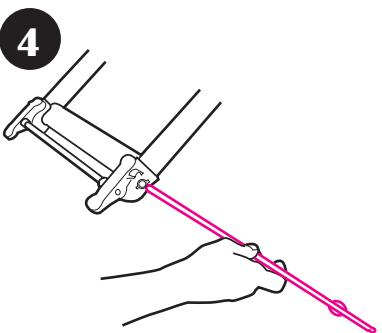
Insert axle rod through axle opening.
