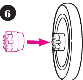
Firmly attach hub adapter onto wheel.
