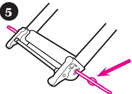
Axle key must line up with key holes.
