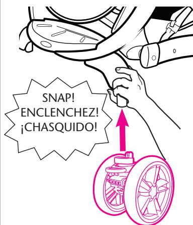
**CHECK** that wheels are securely attached by pulling on wheel assemblies.
