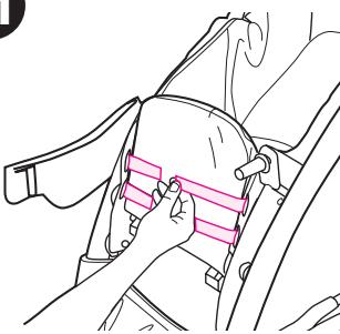
Fasten hook and loop straps together.
