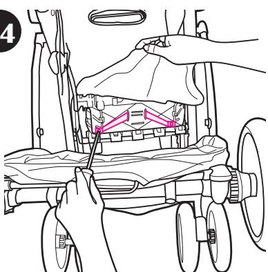
Lift back of seat cover and remove screws on rear of backrest.
