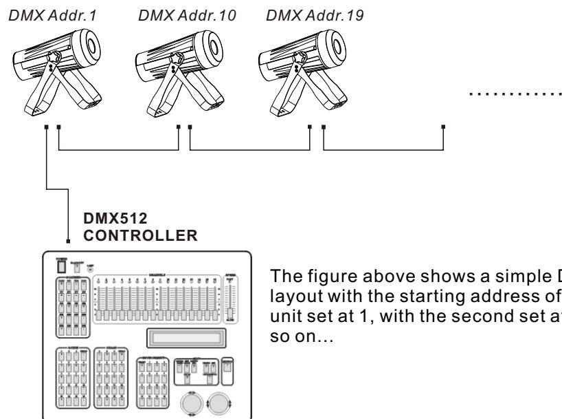
The figure above shows a simple DMX512 layout with the starting address of the first unit set at 1, with the second set at 10 and so on...
