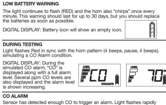
and horn sounds loudly (repeating 4 beeps, pause). See "If Your CO Alarm Sounds" for details. During an alarm, move everyone to a source of fresh air. DO NOT move the CO Alarm!
