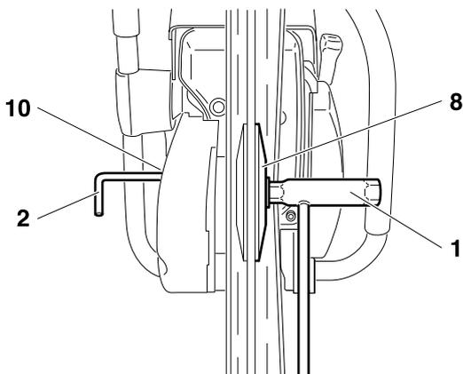
Place the spring washer (8) on the arbour and insert the screw (9) and tighten by hand.
