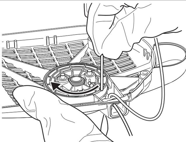
Guide the cable into the recess (24) on the cable drum and use the cable to turn the drum two turns in the direction shown by the arrow.
