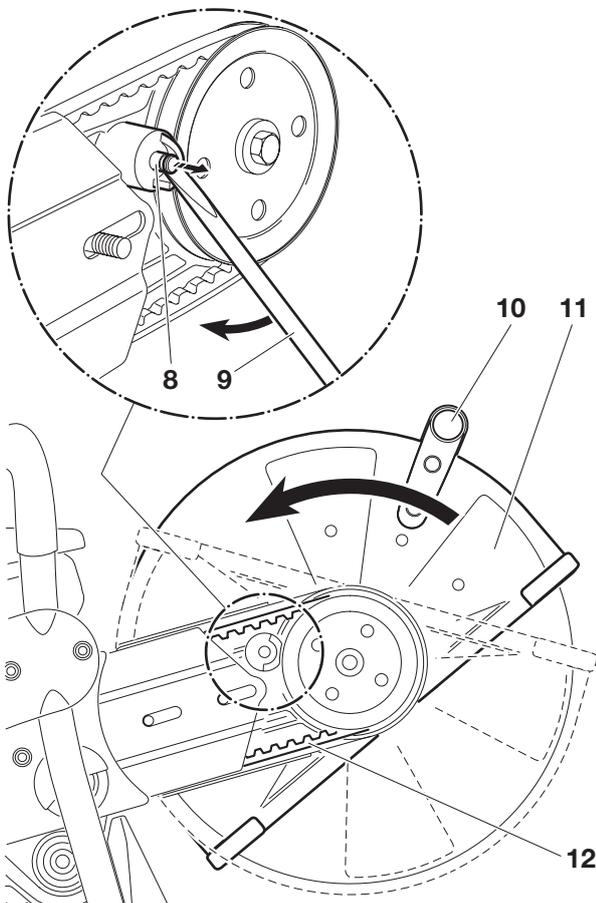
Use the combination tool (8) to lever out the stop pin (9) as shown in the illustration, until the protective hood (11) can be turned.
