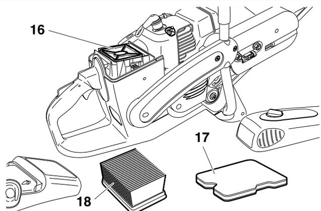
**CAUTION:** Turn off the engine before cleaning the air filter! Never clean out the air filter with compressed air! Do not clean the pre-filter and inner filter with fuel.
