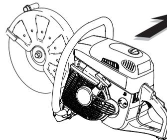
Move the protective hood (3) into the proper position for the work you intend to do (see illustration).
