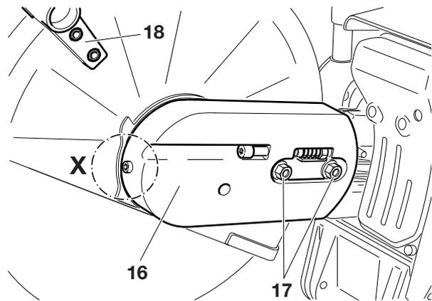
**Replacing/cleaning the spark arrester screen**
