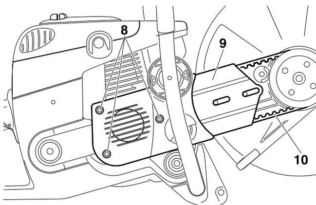
Unscrew the screws (8) and remove the crankcase housing cover (9).
