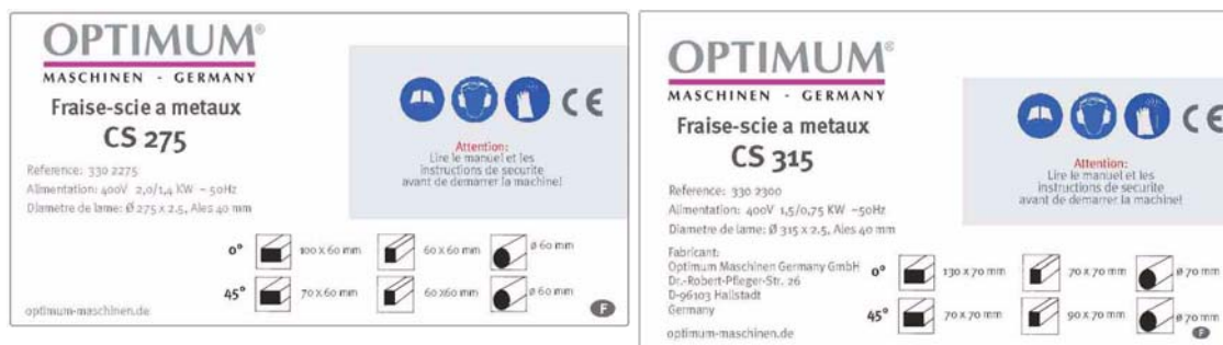
Illustration: 2-1: plaque signalétique CS 275/ CS 315
