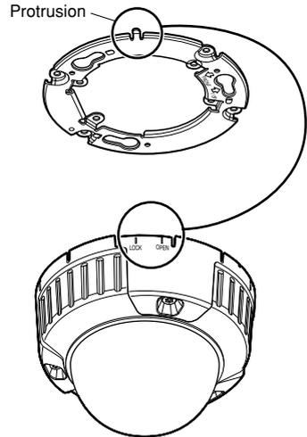
Engage the camera with the camera attachment.
