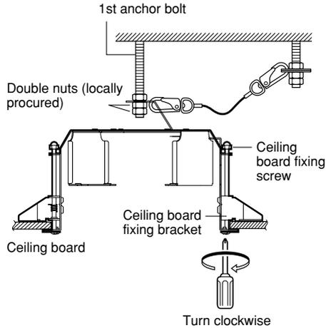
**7. Use double nuts (locally procured) to secure the mount bracket after inserting the 1st anchor bolt.**
