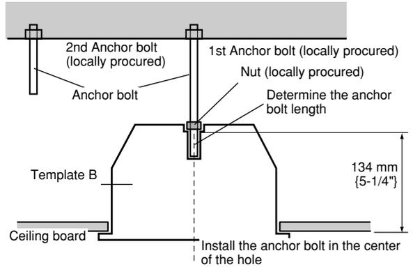
**Note:** If there is already an anchor bolt installed, the anchor bolt can be used as a 2nd anchor bolt. Make sure that the distance between the 1st and 2nd anchor bolts is 1 000 mm {3.28'} or less before use.
