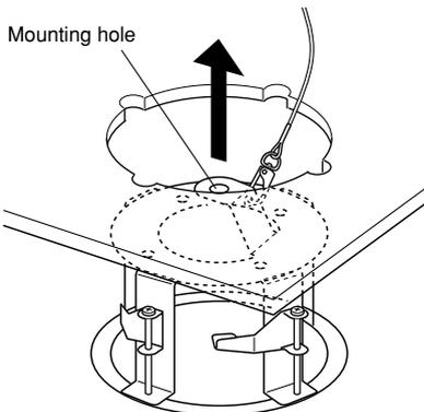
**6. Secure the mount bracket to the ceiling board with the ceiling board fixing screws (4 positions).**
