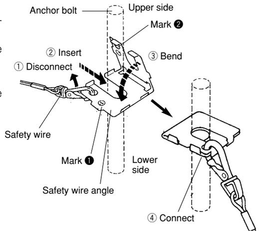
**Note:** To use the anchor bolt that was already installed, the use of 2 spacer nuts (locally procured) is helpful.
