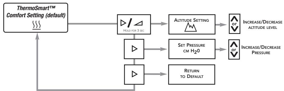
NOTE: Manual adjustment of altitude is not featured on units where there is the Automatic Altitude Adjustment/Leak Compensation feature
