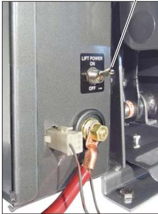
**Lift Power ON/OFF Switch:** This switch must be in the ON position in order to activate the lift controls. The green Power Indicator Light mounted on top of the pump module illuminates to signal power to the lift.
