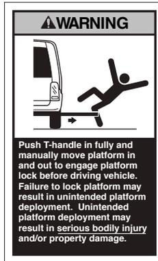
fully extended manually, it does not activate the proper switches for normal operation. Returning (moving) the lift in fully in allows for proper switch activation.
