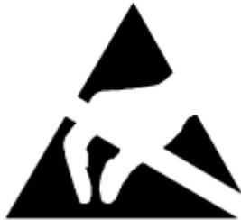
Figure B-1 Electrostatic sensitive devices
