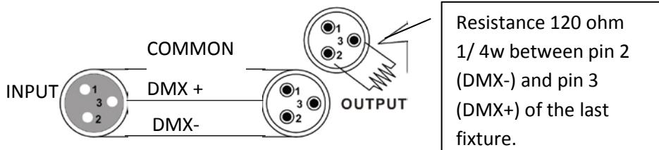
Termination reduces signal errors. To avoid signal transmission problems and interference, it is always advisable to connect a DMX signal terminator.
