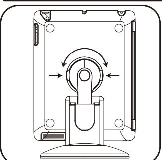
Attach, press and release, spin it to secure it's in position
