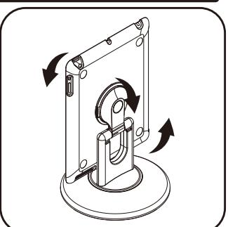
Rotates 360°,tilts for angle adjustment, and reversible view
