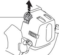
**Primer bulb:** Press the air purge repeatedly until fuel begins to fill the bulb. The bulb need not be completely filled.
