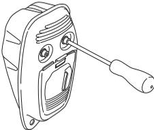
If the muffler on your machine is fitted with a spark arrestor screen this must be cleaned regularly. A blocked
