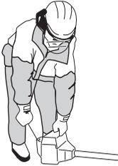
**CAUTION!** Do not put any part of your body in marked area. Contact can result in burns to the skin, or electrical shock if the spark plug cap has been damaged. Always use gloves. Do not use a machine with damaged spark plug cap.
