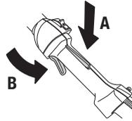
Make sure the throttle control is locked at the idle setting when the throttle lockout is released.
