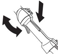
See instructions under the heading Start. Start the machine and apply full throttle. Release the throttle and check that the cutting attachment stops and remains at a standstill. If the cutting attachment rotates with the throttle in the idle position then the carburettor idle setting must be checked. See instructions under the heading Maintenance.
